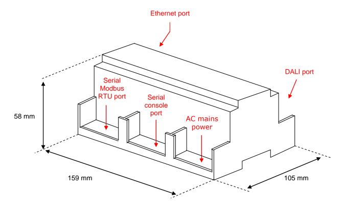
Free space recommended in the install location of the device, with spacing enough for external connections.
