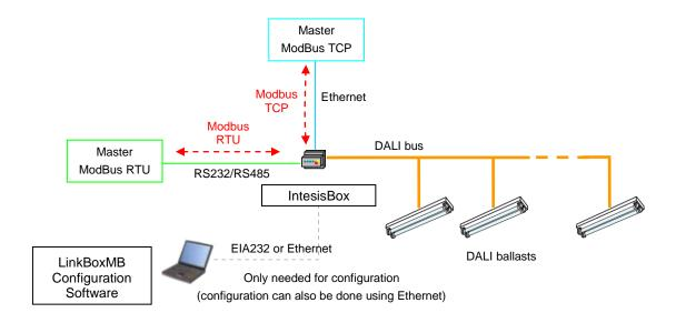
IntesisBox is a DALI master device, monitoring and controlling DALI ballasts connected to a DALI bus (up to 64 ballasts can be integrated within a single channel). IntesisBox also supplies the necessary power for the DALI Bus.
